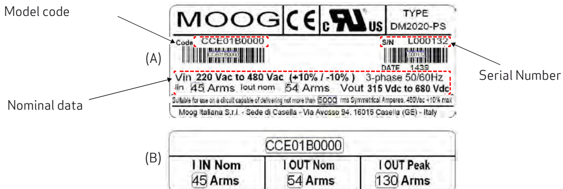
Fig 2.2 Example of power supply side plate (A) and front plate (B)
