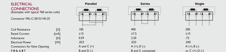
Note: Before applying electrical signals the pilot stage has to be pressurized.
