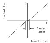
Normally used in failsafe applications
