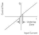
Normally used in hydraulic motor applications
